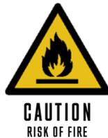
This symbol alerts you to take care as this appliance contains a flammable refrigerant (isobutane) and insulation blowing gas (cyclopentane). Do not expose it to high heat, sparks and open flames.
