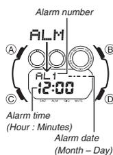
You can set up to three independent multi-function alarms with hour, minutes, month, and day. When an alarm is turned on, the alarm tone sounds when the alarm time is reached. One of the alarms is a snooze alarm, while the other two are one-time alarms.
