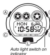
An LED (light-emitting diode) illuminates the face of the watch for easy reading in the dark. The watch's auto light switch turns on illumination automatically when you angle the watch towards your face.
