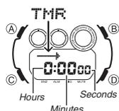
The countdown timer can be set within a range of one minute to 24 hours. An alarm sounds when the countdown reaches zero. The countdown timer also has an auto-repeat feature and a progress beeper that signals the progress of the countdown.
