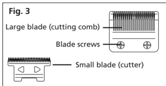
2. To realign the blades, simply match them up, point to point. The top edge of the large blade should be 0.5mm to 1.2mm higher than the top edge of the small blade (see Fig.4). This is important so that the clipper does not cut too close, or come into contact with the skin.
