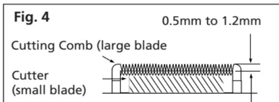
3. The extreme left-hand tooth of the large blade must cover or be to the extreme left hand of the first small tooth on the small blade. Be sure that the extreme right-hand tooth of the large blade touches the extreme right-hand tooth of the small blade.
