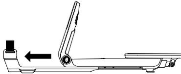
**STEP 5.** Fold out the search coil to detect parallel with the ground (refer to Detecting Basics). Tighten the wing nut to fix the coil position. Be careful not to over tighten.
