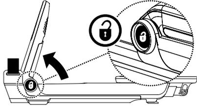
Failure to press the unlock button when releasing handle will cause damage.
