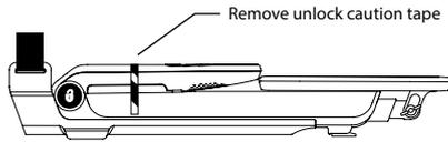
**STEP 2.** Press down the red UNLOCK button on both sides to release the handle.
