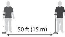
**SPACE** Recommended distance is 50 feet (15 m) apart when multiple users are scanning an area.
