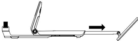
To retract shaft, firmly tap on the base of the coil.
