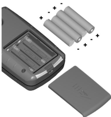
Be certain to align the batteries as per the diagram within the battery compartment.
