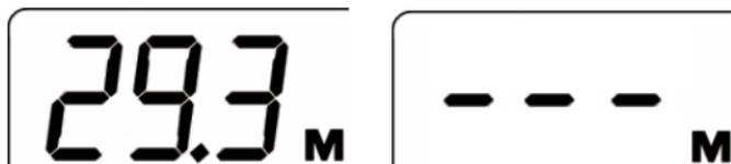
The depth readout on the top left, will appear after the power is turned On and the transducer is placed in water.
