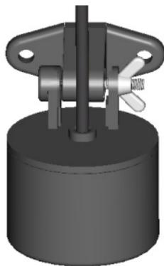
**3** Your Fish Finder includes a combination adapter, mounting bracket for the sonar sensor. The Adapter includes mounting taps so that you can attach it to any flat surface or boat hull and appropriate rod, The Adapter is removable and adjustable up to 180 Degrees.
