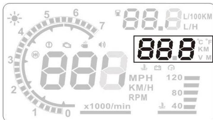
Pull the button downward for 5 seconds to turn off the alarm buzzer, and the icon will disappear. Push the button upwards for 5 seconds to turn the alarm buzzer on, and the icon will appear.
