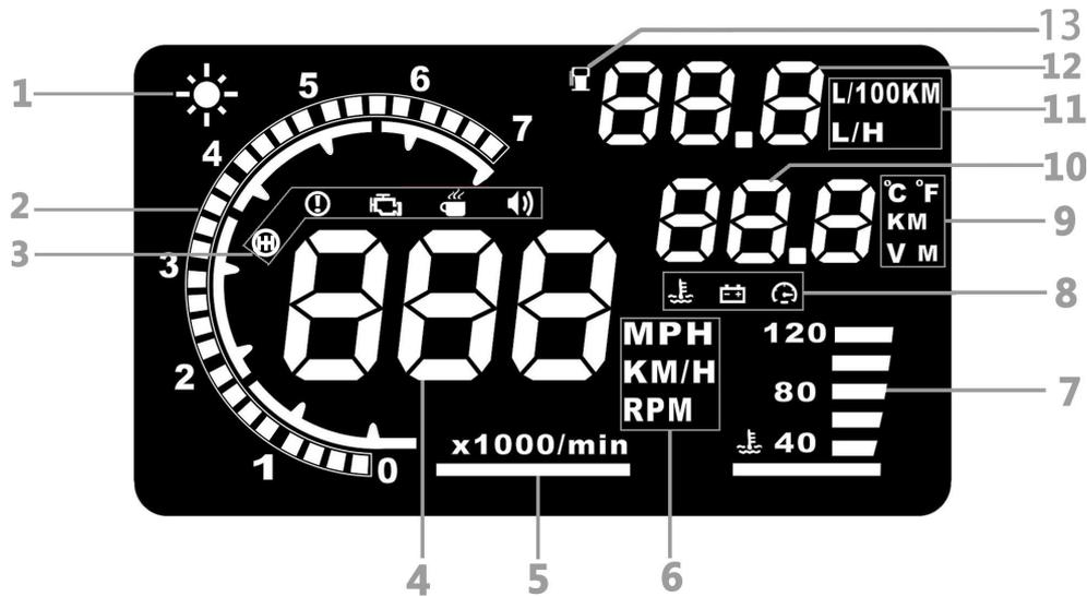
1. **Light Sensor:** changes the unit display brightness to suit the environment
