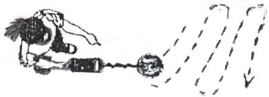
If there is a sound of “di-di” during moving, it indicates that there is a metal target in the sound area. In this case, you can use “TARGET PINPOINTING” to pinpoint the target. Then use “DISC” or “DISC/TONE” to determine whether the target is worth digging out. The followings are the four operation modes in detail.
