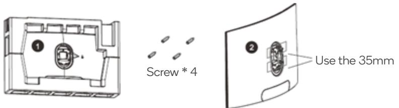
4. Follow the directions received with your mount, stand or accessory and install the monitor on the wall or fixture as desired.
