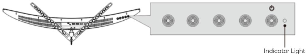
Solid blue light indicates power is on and the monitor is operating normally. Flashing blue light indicates no video source no horizontal or vertical signal has been detected.
