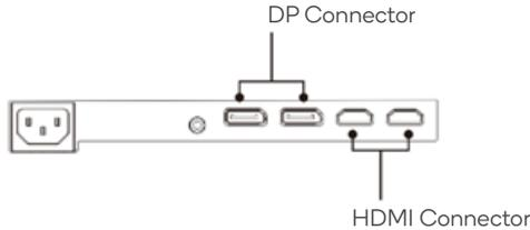
2. Connect the power cable to your monitor then connect the other end to your power source. It is recommended that you use a surge protector with adequate voltage if a wall outlet cannot be reached directly.
