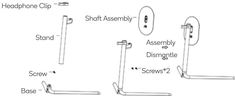
2. Remove the monitor from the carton, lay it flat with the back facing upwards and clamp the base assembly to the rotating shaft of the monitor.
