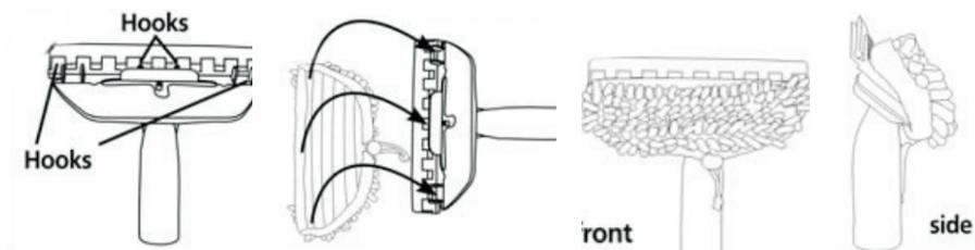
2. Attach the window cleaning tool to the extension hose as follows:
