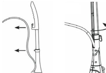
2. Unlock the button on the extension hose and take out the hand-held steamer.
