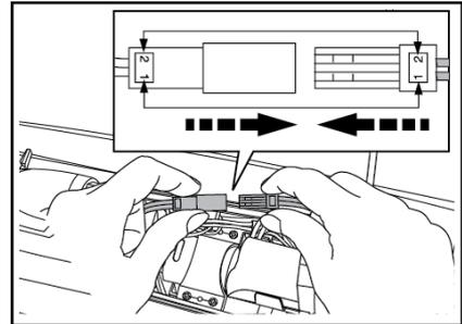
Connect the socket of the rechargeable battery pack as shown above.
