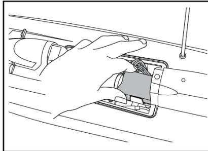
Place the rechargeable battery pack in to the bracket at the rear area of the boat hatch and stick it in with the magic sticker tightly. Ensure it is secure.
