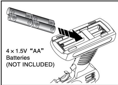
Remove the battery cover on the controller. Place 4 x AA batteries into the battery compartment, noting the correct polarities. Replace the battery cover.
