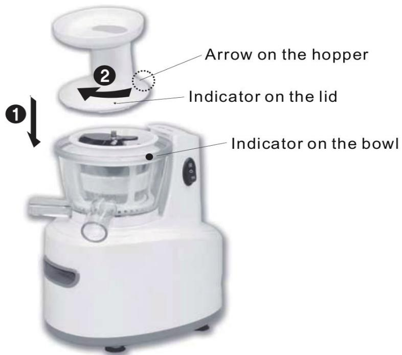
4 – Assemble the hopper onto the bowl.
