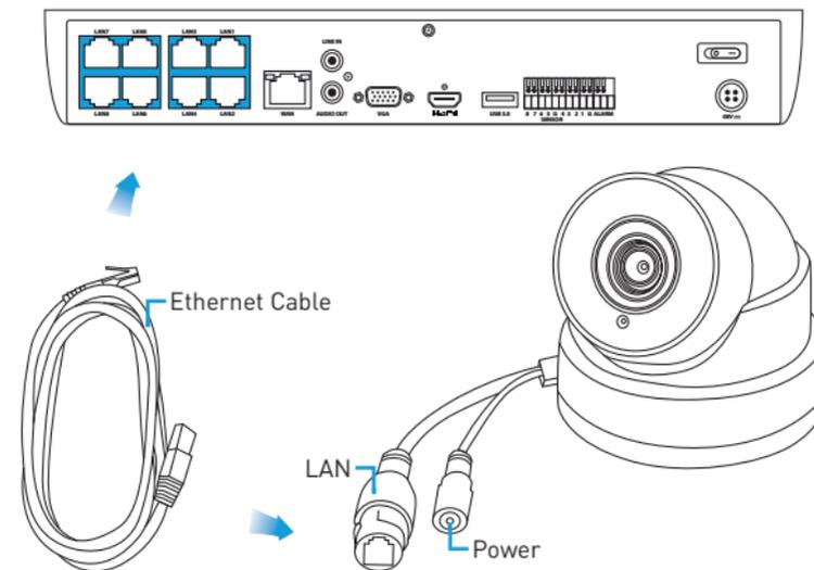
**Please note:** The power connector is provided as an alternative power option if required. Your NVR will provide power over the Ethernet cable when connected and a separate power adapter is not required.
