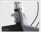
**Step Four**: Unlock the handle post latch by pulling it away from the handle post.
