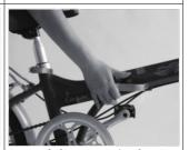
Step Eight: Move the frame safety hook to the open position.
