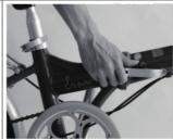
**Step Three**: Lock the frame latch lever by pushing it towards the frame.
