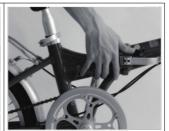
**Step Four**: Move the frame latch safety hook into the closed position.
