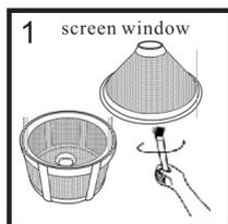
Take out the safety net. Clean the mosquito trap from the bottom to the top. Firstly turn the base anti-clockwise and separate unit. Take out the **screen window rubber**, then pull out the **screen window**, and clean the screen window with a brush, as shown to the left.
