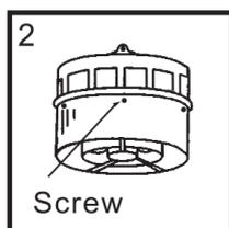
Taking the central fan section, unscrew the screws that are situated around the unit, then separate the two sections from each other.
