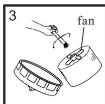
Clean the inside of the central fan unit with the brush. You may also wipe the sections down with a piece of wet cloth.
