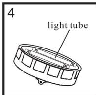
Remove the top light section and lay it upside down. Give the light tubes a half turn, at which point they can be lifted out. Press the new replacement tubes into the slots and give a half turn in the opposite direction to lock it into position.
